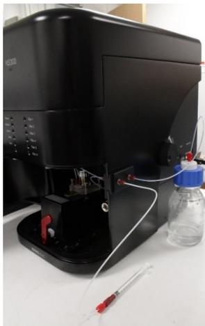
**Figure 5-15:** External NS300 fluidic connections.
