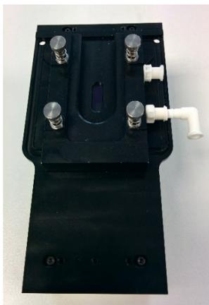
**Figure 5-10:** O-Ring top-plate.
