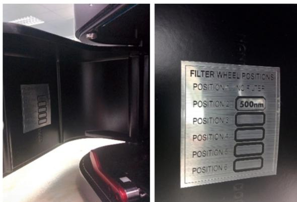
Fluorescence filters are mounted on an integrated filter wheel within the instrument housing. Introduction of filters into the optical path is controlled by the NTA software. The position of filters installed in the filter wheel is displayed on a sticker inside the access hatch for each NS300 system.
