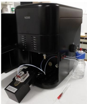
**Figure 7-1:** Loading a sample with the LVFC.
