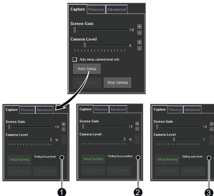
Figure 8-13: Auto-setup for fully automated capture settings.
