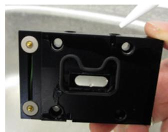
**Figure 12-9:** Cleaning the O-Ring top-plate.
