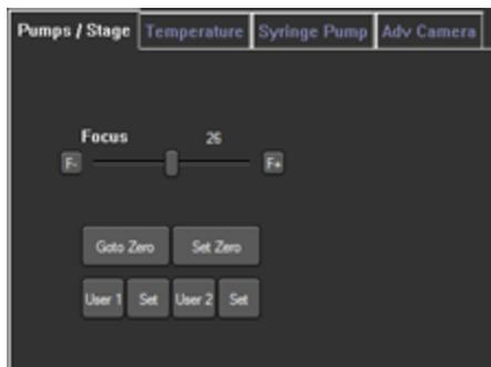
**Figure 8-10:** Fine focus adjustment in the NTA software.
