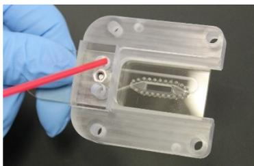
A: Drying gasket component through manifold tubing ports
